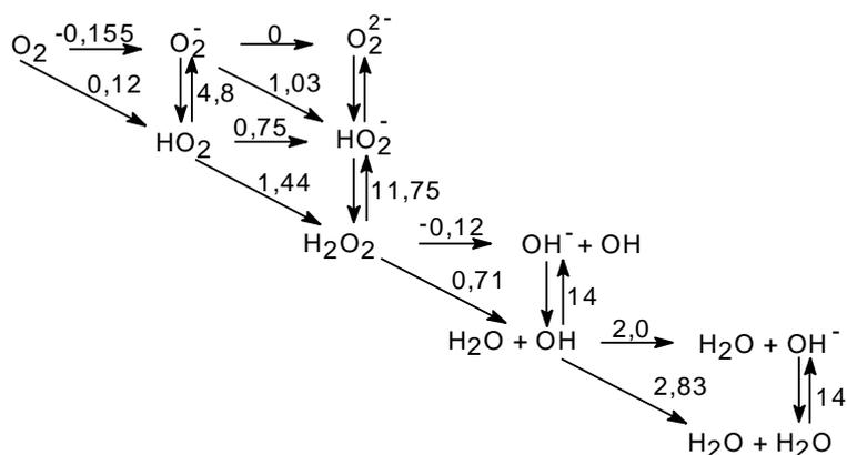
Figure 2. Activation of oxygen molecule with the intermediate formation of  $H_2O_2$  [10].
