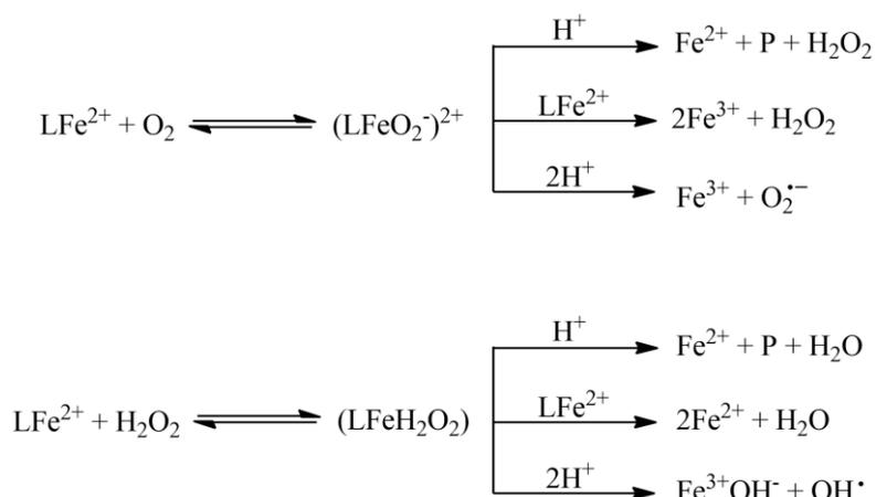
Figure 6. The mechanism of O<sub>2</sub> activation with iron coordination compounds [10].
