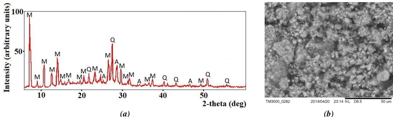
Figure 1. The X-ray diffraction pattern of Nakhchivan zeolitic tuff\* (a) and its SEM image (b). \*(M – mordenite, Q – quartz, A – anorthite)
