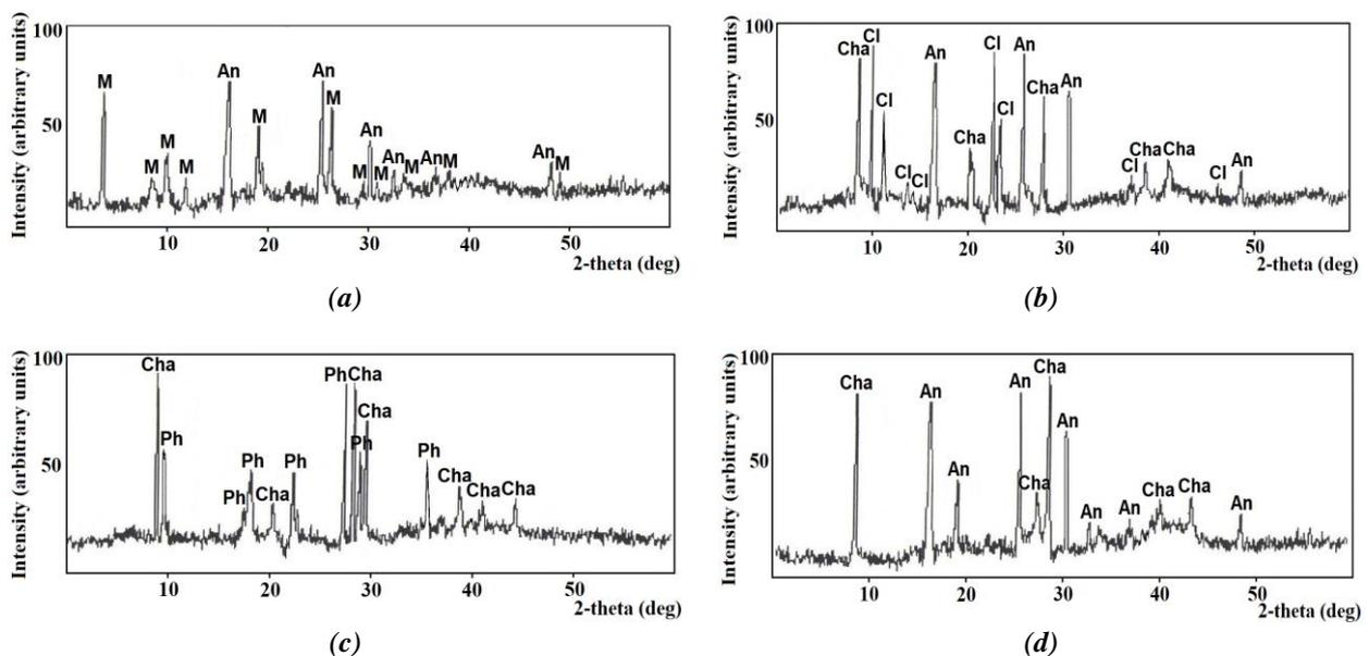
**Figure 4. X-ray diffraction patterns of crystallization products\* obtained in: KOH+KCl at 150°C for 50 hours (a); KOH+KCl at 200°C for 80 hours (b); KOH+NaOH at 150-200°C for 50 hours (c); KOH+NaOH+KCl+NaCl at 200°C for 80 hours (d).**
