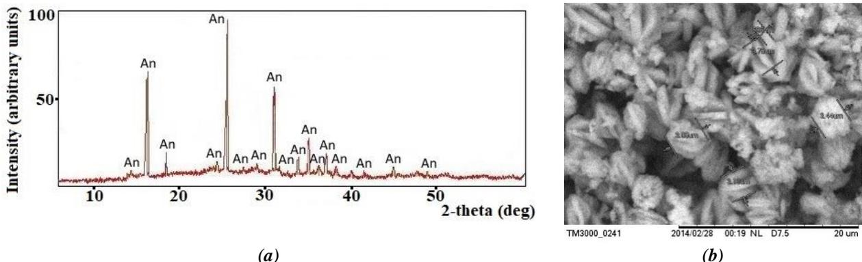
Figure 2. The X-ray diffraction pattern of analcime (An) with 100% degree of crystallinity (a) and its SEM image (b).
