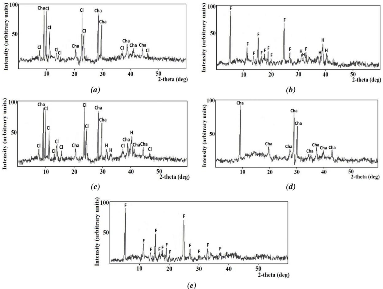
**Figure 5.** X-ray diffraction patterns of crystallization products\* obtained in: 20% KOH and 15% KCl (a); in KOH+KCl at 30% KOH (b); at 30% KOH+NaOH (c); in KOH+NaOH+KCl+NaCl at 20% KOH+NaOH and 15% KCl+NaCl (d); in KOH+NaOH+KCl+NaCl at 30% KOH+NaOH (e).
