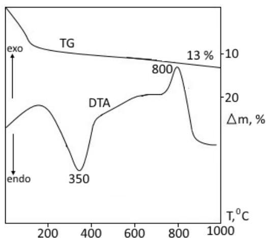
**Figure 3.** Thermogram of synthesized analcime zeolite obtained under optimal conditions.
