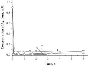
Figure 6. The concentration of  $Ag^+$  ions in the *Vitex* extract + AgNO<sub>3</sub> mixture versus time of the reaction at  $40^{\circ}$ C (1),  $60^{\circ}$ C (2) and  $80^{\circ}$ C (3).
