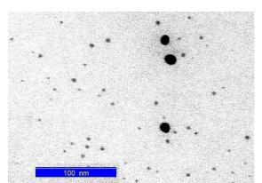
Figure 5. TEM image of the *Vitex* extract + AgNO<sub>3</sub> mixture stirred at 80°C during 5 h.
