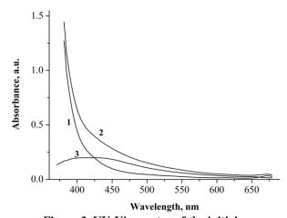
Figure 3. UV-Vis spectra of the initial Vitex extract + AgNO<sub>3</sub> mixture (1), of the mixture, stirred at 40°C during 48 h (2) and the difference between these two spectra (3).
