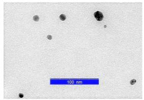
Figure 4. TEM image of the *Vitex* extract + AgNO<sub>3</sub> mixture stirred at 40°C during 24 h.
