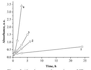
Figure 2. Absorbance at the maximum of SP resonance band in the UV-Vis spectra of the Vitex extract + AgNO<sub>3</sub> mixtures versus time of the reaction at 50°C (1), 60°C (2), 70°C (3) and 80°C (4).
