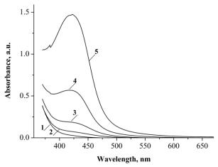
Figure 1. UV-Vis spectra of the initial *Vitex* extract + AgNO<sub>3</sub> mixture (1) and of the mixtures stirred at 80°C during 0.75 (2), 1.5 (3), 3 (4) and 5 h (5).
