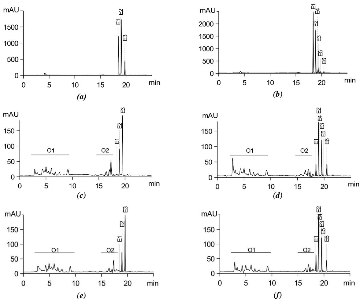
Figure 4. Chromatograms for initial BD1 (a) and BD2 (b) biodiesels, for oxidized BD1<sub>ox</sub> (c) and BD2<sub>ox</sub> (d) samples, and for oxidized (BD1+AOs)<sub>ox</sub> (e) and (BD2+AOs)<sub>ox</sub> (f) samples.
